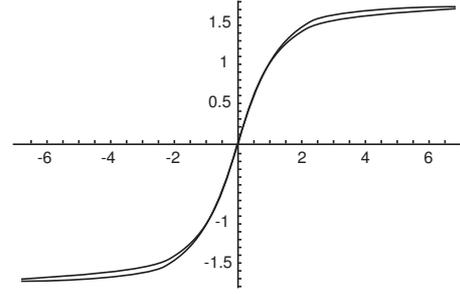
**Figure 6.** The popular hyperbolic tangent activation function  $y \leftarrow 1.7159 \tanh(\frac{2}{3}y)$  can be approximated by a pair of circular nodes where the activation of the second node  $y_q$  is fixed at  $\sqrt{1.9443}$  and the activation of the first node is calculated accordingly  $y_p \leftarrow 1.7159 y_q / \sqrt{y_p^2 + 1.9443}$ .
