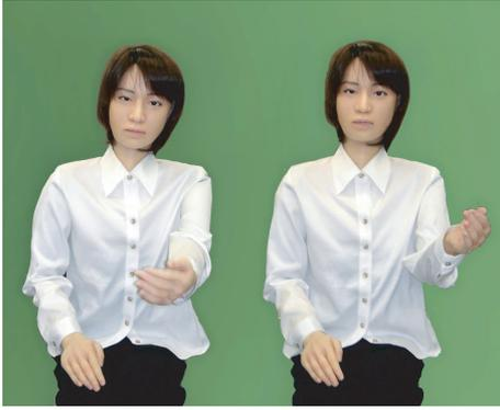
**Figure 2.** Actroid, the actress android, has 33 motors, which are driven by compressed air, to move its head, neck, arms, body, eyes, eyelids, and mouth. Actroid can make smooth and natural movements, including large and small gestures. Actroid has touch sensors in the arms and can access floor and infrared sensors and video cameras placed in the environment.
