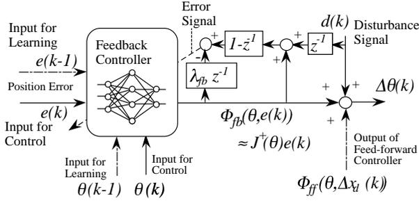
Fig. 4: Learning based on Disturbance Noise and Feedback Error Signal
