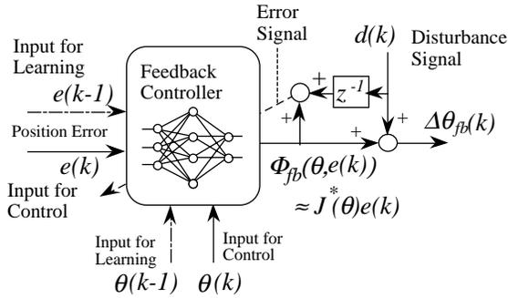
Fig. 3: Learning based on Feedback Error Signal
